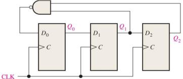
65. Determine the state diagram of the following counter
