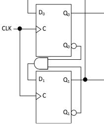
67. Determine the state diagram of the following counter.  $Q_1$  is the MSB.
