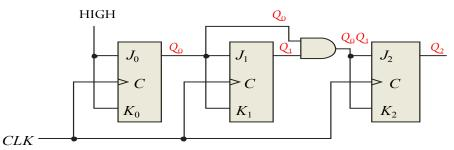
66. Determine the state diagram of the following counter.  $Q_1$  is the MSB.
